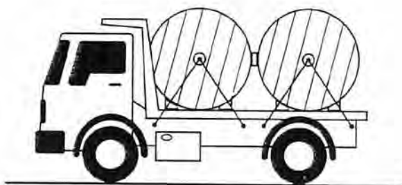
Secure drums adequately before transportation
